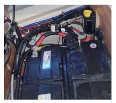
The solar panel (360W) with a 30A charger allows you to keep the services batteries charged on a sunny day, but on a cloudy day and at night the refrigerator must be turned off to avoid discharge less than 12.2v.
