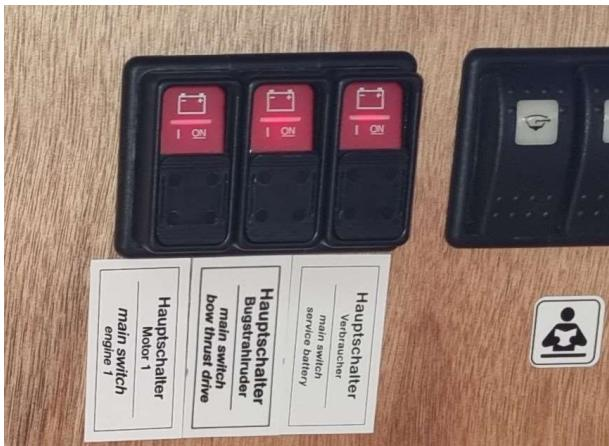
Switch on button for thruster activated
