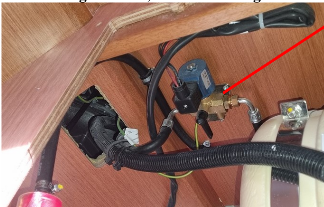
Emergency fuel shut-off (Stbd aft cabin under bunk)
