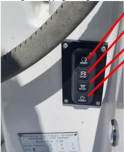
When the button is depressed the pre-heat function is activated and the start motor engaged.
