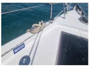
To use the fresh water system, turn on the fresh water breaker on the 12v panel and open a faucet. When a tank runs out of water, the pump will run at high speed and the faucet will start to cough air. As soon as you hear the pump running continuously, check to see if anyone is using water. If not, switch off the pump immediately to prevent the pump from drawing more air into the system or the pump overheating.
