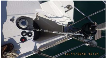
Remove the safety line and push the anchor over the bow, keeping hands and feet clear. Control the rate the chain pays out by tightening or loosening the brake with the windlass handle.
