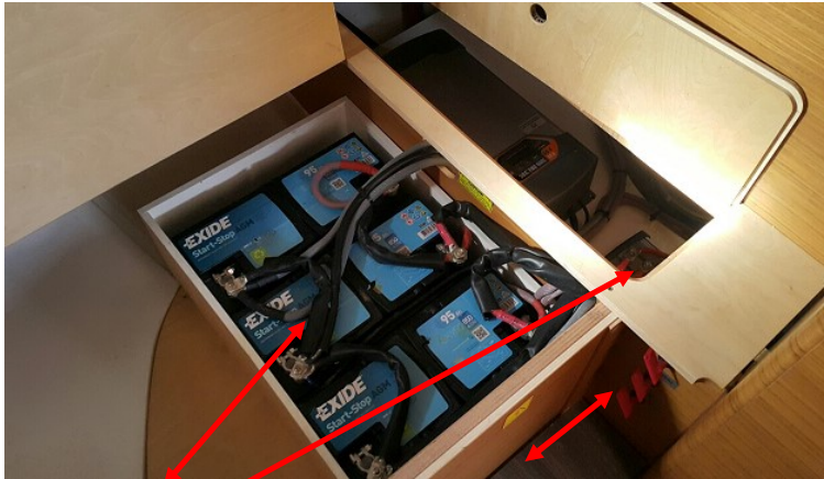
The service batteries ,main breakers with red key, anchor windlass fuse are located on the wall starboard cabin .
