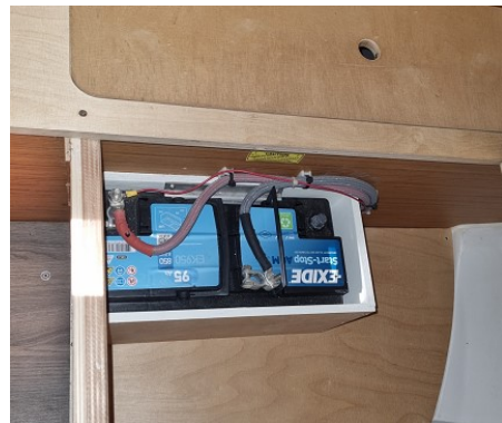
Start battery is located under the bed of aft port cabin
