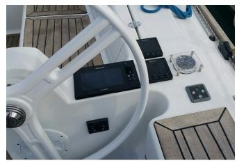
Engine switch on/out; Volvo engine tachometer (max 2200 rpm)
