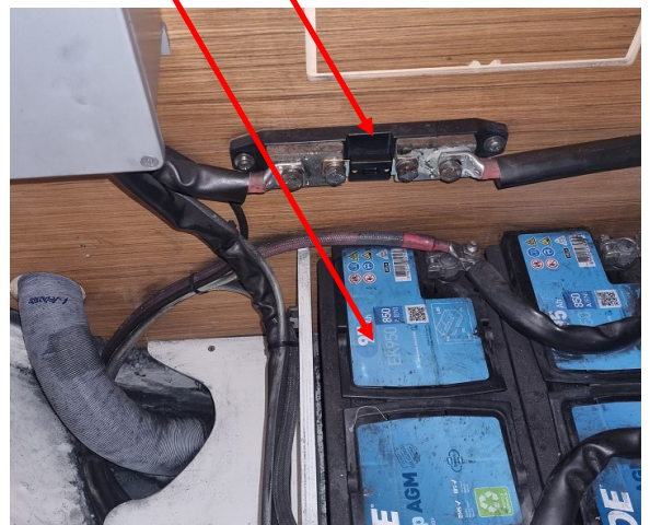
Bowthruster batteries and fuse are located under the bed of bow cabin.
