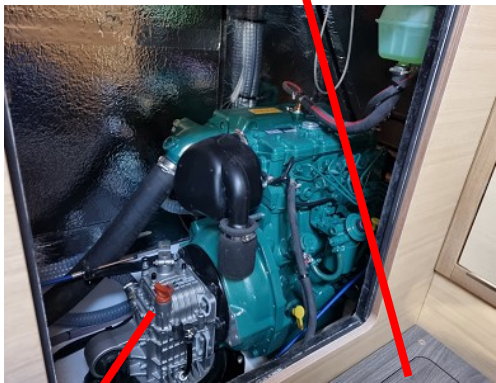
Engine cooling water inlet Gear oil refill and dipstick
