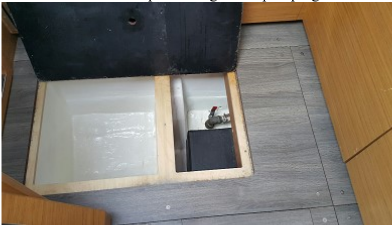
Valve must be open during waste pumping
