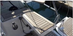
Yacht is equipped with retractable transom (bathing platform) .There is a swim ladder. While under sail, the transom should remain closed and secure. After you have gotten to your anchorage feel free to deploy the transom for easy access to your dinghy, swimming or snorkeling.
